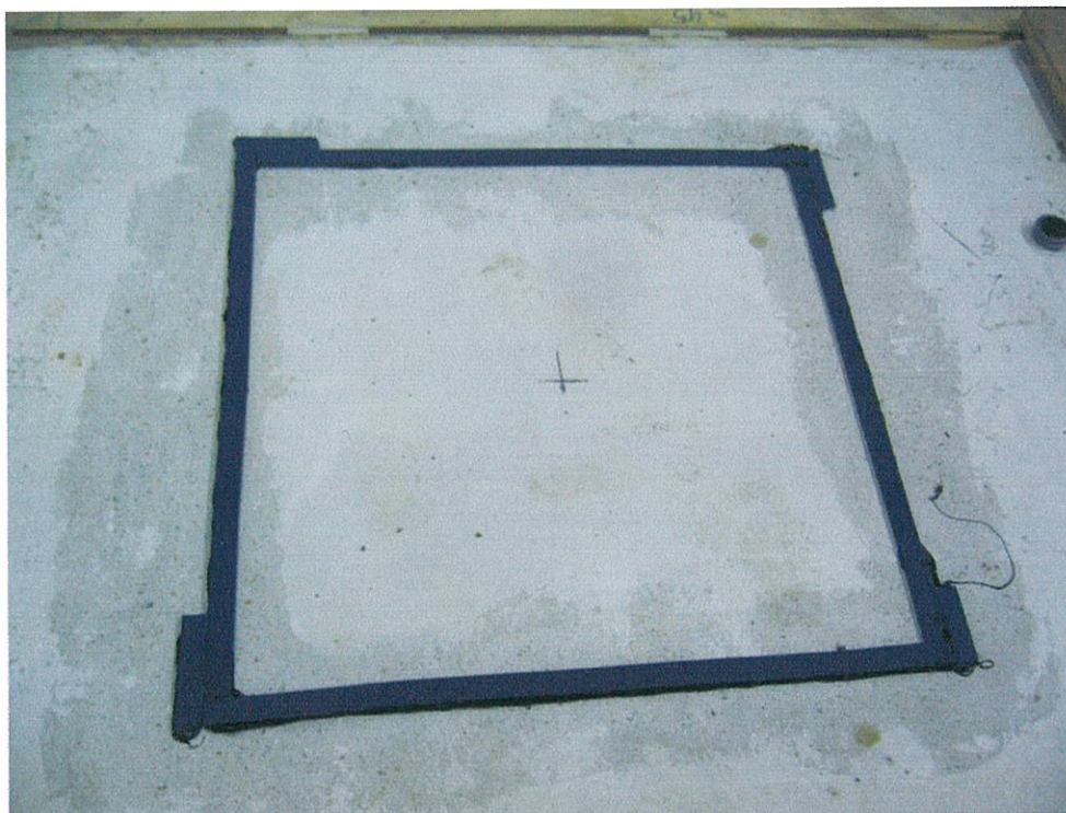
Fig.A2: Specimen with fitted swelling tape
