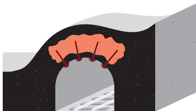
Consolidation and sealing
