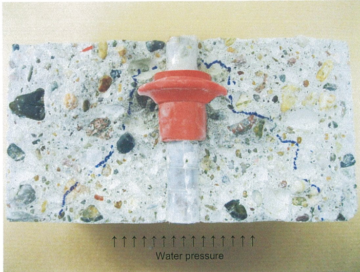
Fig. A2: Sample 1: anchor rod (ribbed steel \text{\O} = 16 \text{ mm} )
