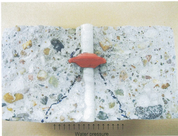
Fig. A3: Sample 2: glass-fibre rod (ribbed \text{\O} = 14 \text{ mm} )
