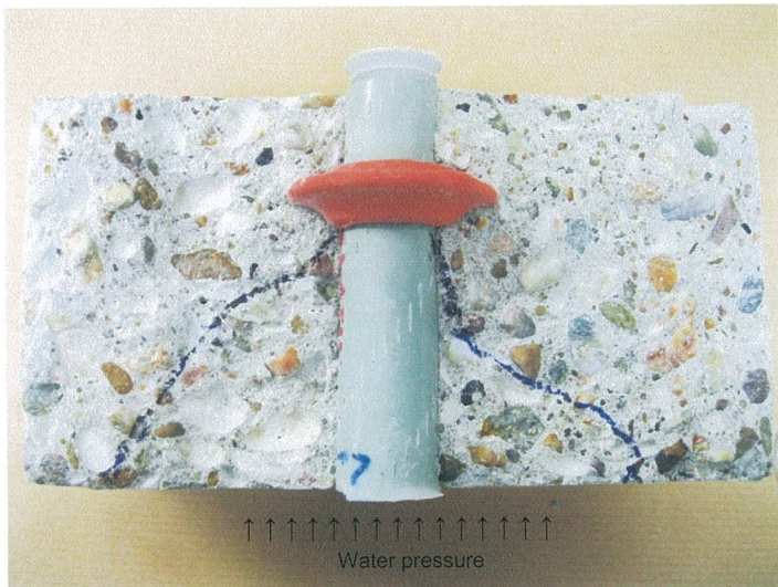
Fig. A5: Sample 4: plastic pipe ( \varnothing_{\text{inside}} = 22 \text{ mm} , \varnothing_{\text{outside}} = 26 \text{ mm} ); negative water pressure acting on the plug
